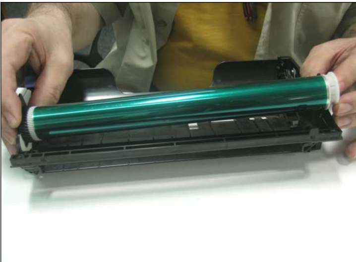
22. When the drum is extracted there will be a spring loaded clutch piece at one end and a drive gear on the other side coming loose.
